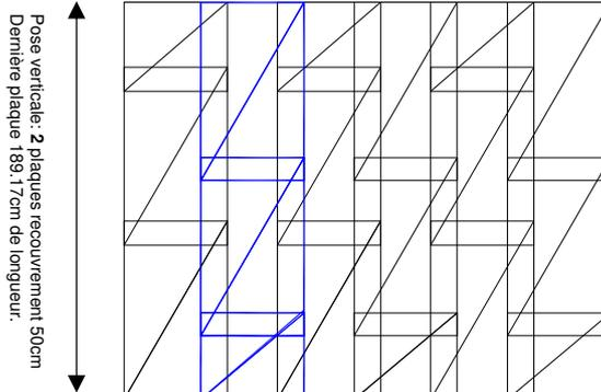
Pose verticale: 2 plaques recouvrement 50cm
