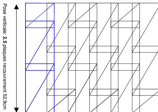
Pose verticale: 2.5 plaques recouvrement 52.9cm
